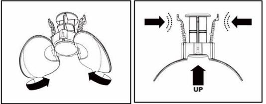
The diagram consists of two panels. The left panel shows the VasoStat device with two paper strips being peeled away from the adhesive wings. The right panel shows the device with the plunger moved to the 'up' position, indicated by a large black arrow pointing upwards and the word 'UP' below it. Dashed lines and arrows indicate the wings being squeezed together to achieve this position. |
